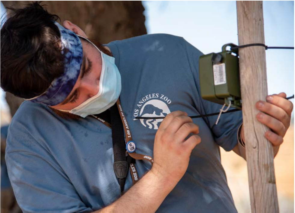
(Above) Conservation Intern, Daniel Chroman installs a wildlife acoustic monitoring system in the Zoo's 6-acre oak woodland area. This monitoring system can collect several weeks' worth of bird sounds and will be utilized as one method of data collection for native wildlife in the Zoo. Photo credit Anna Becker.
